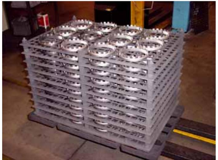
**Fig. 4:** CFC-fixturing for Internal Ring gears
