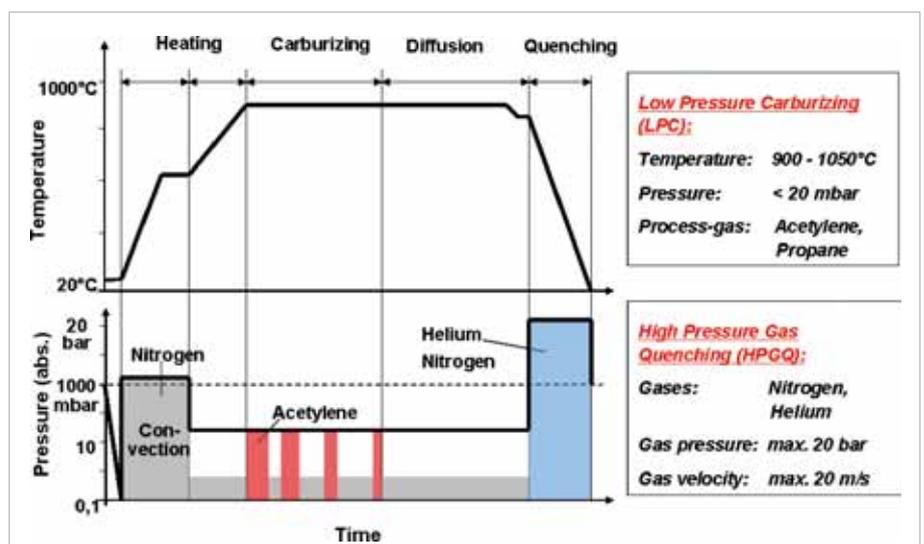
Fig. 1: LPC and HPGQ process (schematic process-cycle)
