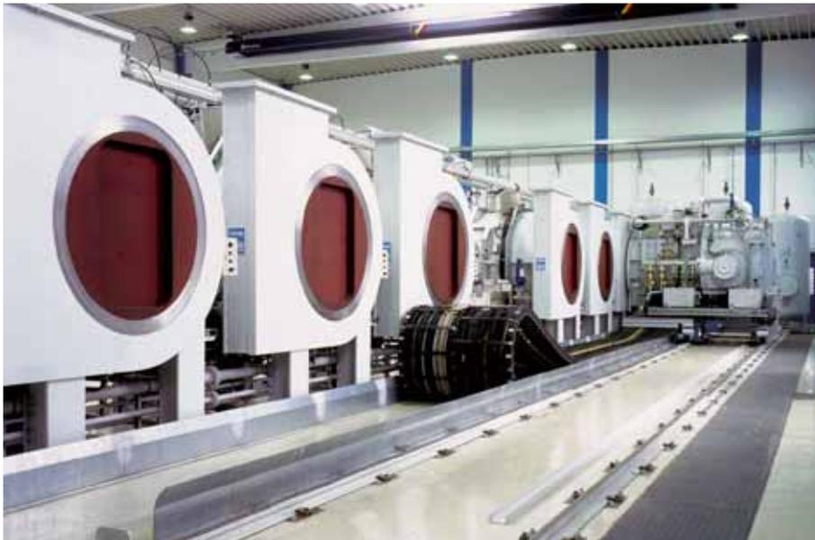
Fig. 2: ModulTherm® plant for LPC and HPGQ process
