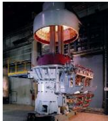
Vacuum crucible preheat station
