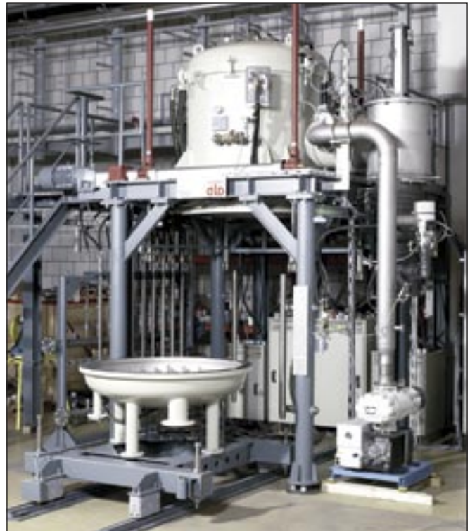
Figure 3—Bottom loader for LPC of large parts with integral gas quench.
