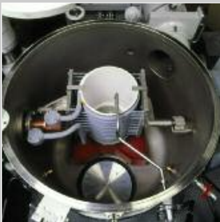
Gas purging with pivotable gas inlet into the melt
