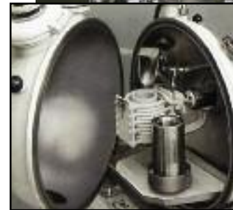
VIM 02 VIM furnace with diffusion pump and cell charger for laboratory use
