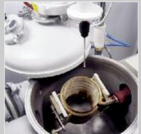
Temperature measurement with thermocouple and reusable protection tube
