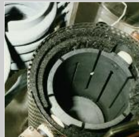
Mold heater keeps the cast liquid and allows subsequent controlled solidification
