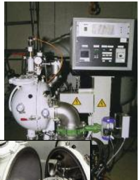
VIM 02 VIM furnace with diffusion pump and cell charger for laboratory use
