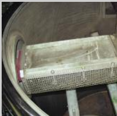
Casting via tundish with heater enables filtering of undesired inclusions and precise pouring stream into e.g. barstick molds
