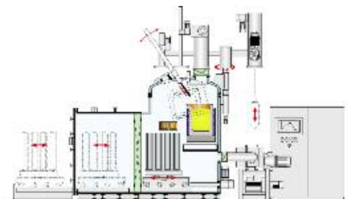
VIM HMC Two Chamber Design with Horizontal Mold Chamber allows to lock in molds prior to casting without interrupting the furnace atmosphere - this avoids excessive temperature losses of preheated molds
