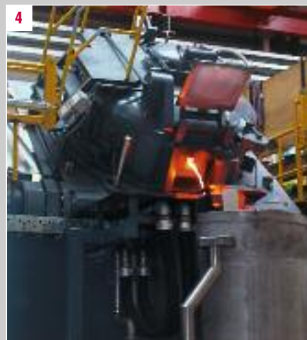
Pouring under protective gas
