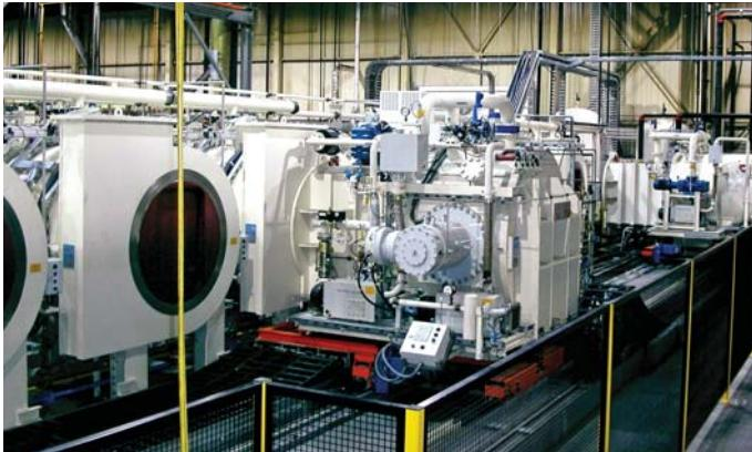
**Fig. 8. ModulTherm® system for vacuum deoiling and carburizing of PM sprockets**
