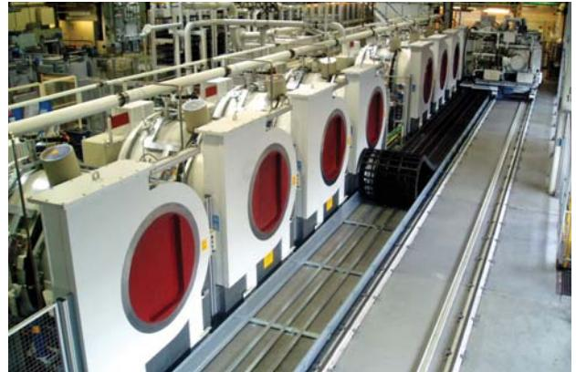
**Fig. 9. Fully automated 8-chamber ModulTherm® for vacuum carburizing and gas quenching of bevel-gear pinions (BMW)**
