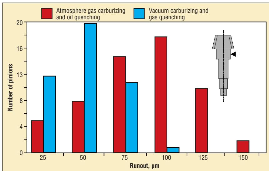
Fig. 5. Reduction of run-out distortion of vacuum-carburized and gas-quenched bevel-gear pinions
