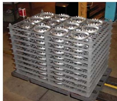
(Left) Fig. 3. Large crown wheels of commercial vehicles. (Above) Fig. 4. Ring gears of 6-speed automatic transmission loaded on CFC grids.
