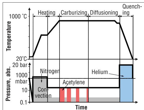
Fig. 2. Schematic process flow
