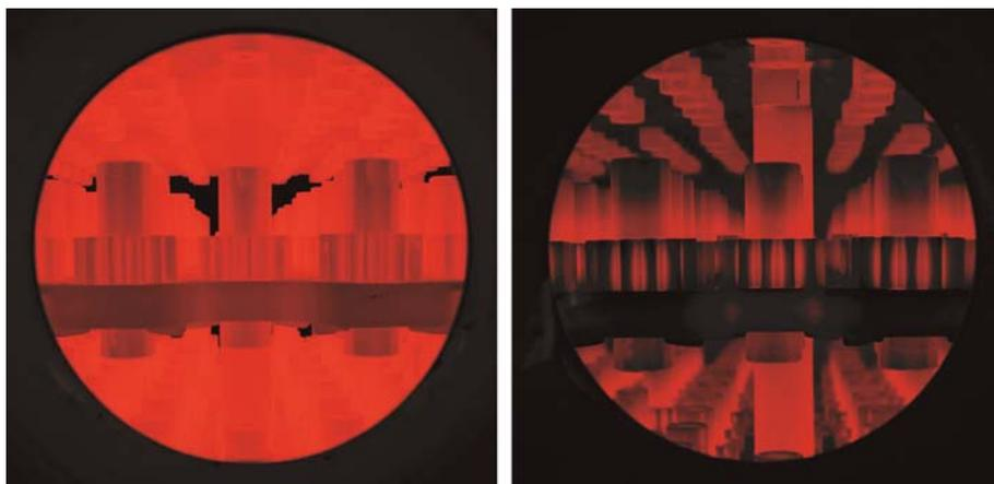
**Fig. 5:** Gas quenching of a load of gear parts in the cold quenching chamber of DualTherm® a) shortly after the start of the gas circulator and b) 5 s later
