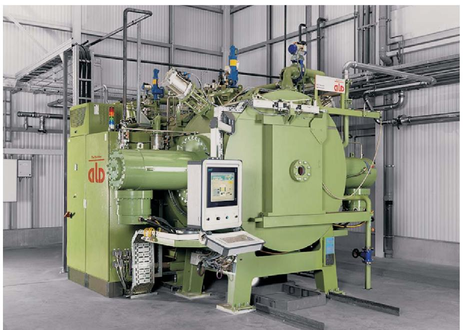
Fig. 1: Dual chamber vacuum furnace, type DualTherm®
