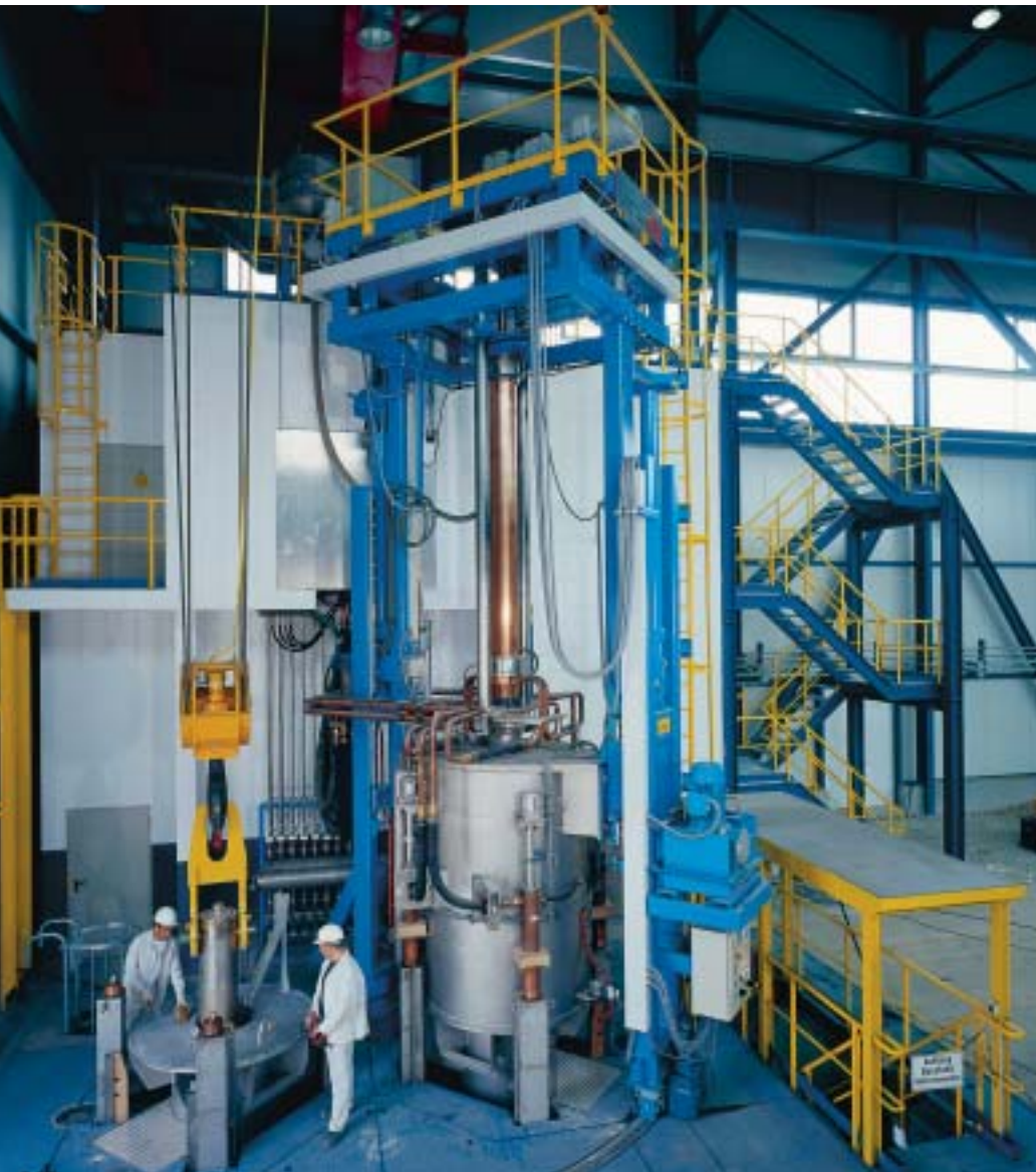
20 ton ESR furnace capable of melting under protective atmosphere.
